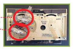
Please recycle the whole thermostat, do not remove mercury switch
